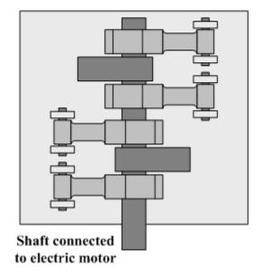
The principle of this type of fatigue test rig is based on inertia forces generated by out-of-balance shaft.
